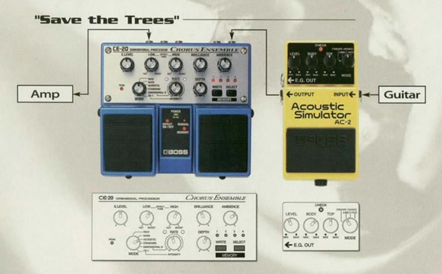
Turn your electric guitar into a deep-bodied acoustic-electric with the AC-2 Acoustic Simulator's "Jumbo" setting. Then, for a rich, warm chorus sound, plug into the CE-20 Chorus Ensemble and set it for "Acoustic Chorus". The CE-20's Ambience and Brilliance switches add the necessary rich chorus and subtle reverberation along with some high-end sparkle. You can add more depth to your tone by turning up the Ambience. Try this setup and save a tree!
